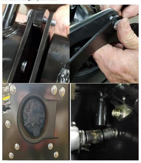
Install you (4) 30-0051 Nuts onto the bolts that you hung earlier in the process and tighten.
