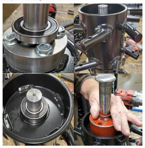
Mount the 40-0475 1" 3 Bolt Flange Bearing to the 10-3303 Center Bearing Plate using (3) 30-0374 Carriage Bolts and (3) 30-0051 Flange Nylock Nuts.
