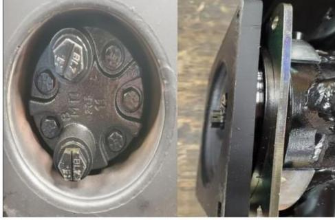
Once aligned place (4) 30-0411 Carriage bolts in to hold it in place.
