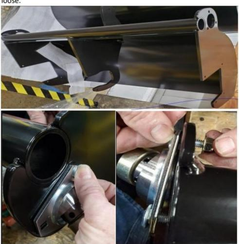
Slide the Carbon Fiber Rod through both of the Bearing for alignment. Tighten the nuts.
