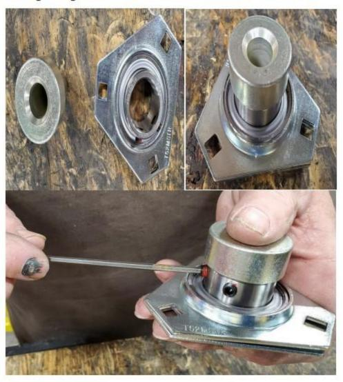
Install the Bearing onto the 20-3300 Tine Drum Housing on both sides using (6) 30-3340 Carriage Bolts leaving the (6) 30-0051 Nylock Nuts loose.
