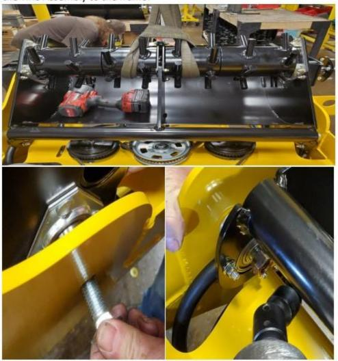
Lift the Assembly up and place a 2\*4 in between the Drum Assembly and the Frame and Lower.
