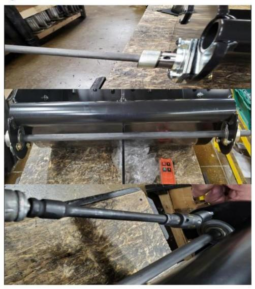
Using the strap, rig the Drum Assembly as shown.
