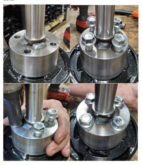
Slide the 40-1423 1" Deep Groove Caster Bearing over the Float Shaft.
