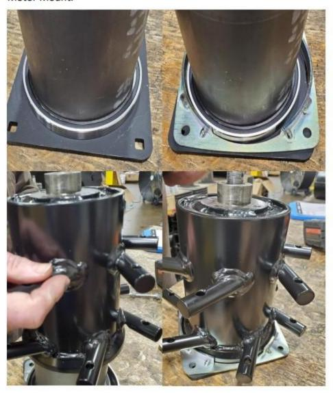
Place the Castle Nut back onto the Tine Motor Shaft.
